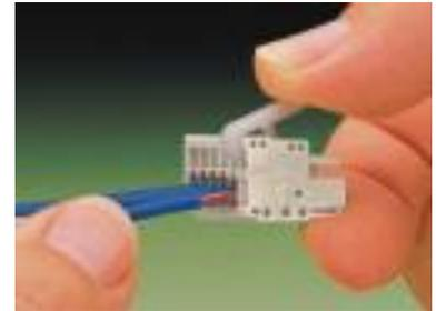
Pulled off spring terminal with operation tool:
