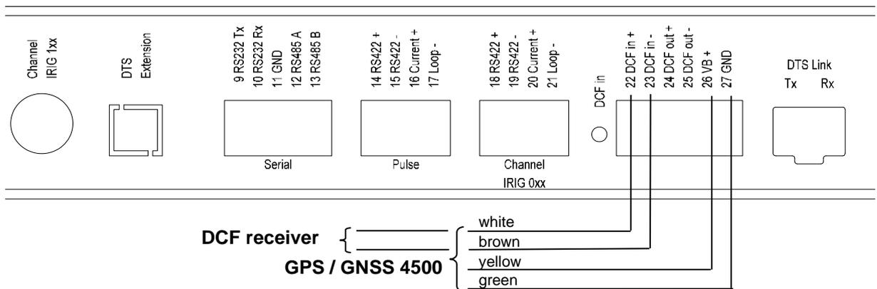
GNSS 3000 according to manual Bx-800813 chap. 9.2 Connection schematics DCF current loop
